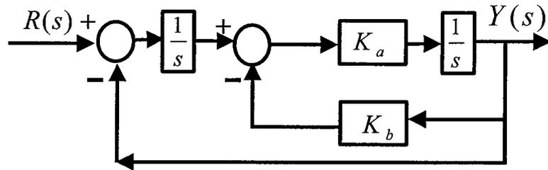
A design specification is that the closed-loop poles of the system are located at the following given positions in the s-plane.
