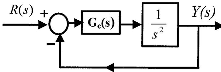
Design a phase-lead compensator  $G_c(s)$  such that the closed-loop compensated system has a time constant  $\tau=0.5$  s and a damping ratio  $\zeta=0.707$ . The compensator has a dc gain as  $8/3$ .
