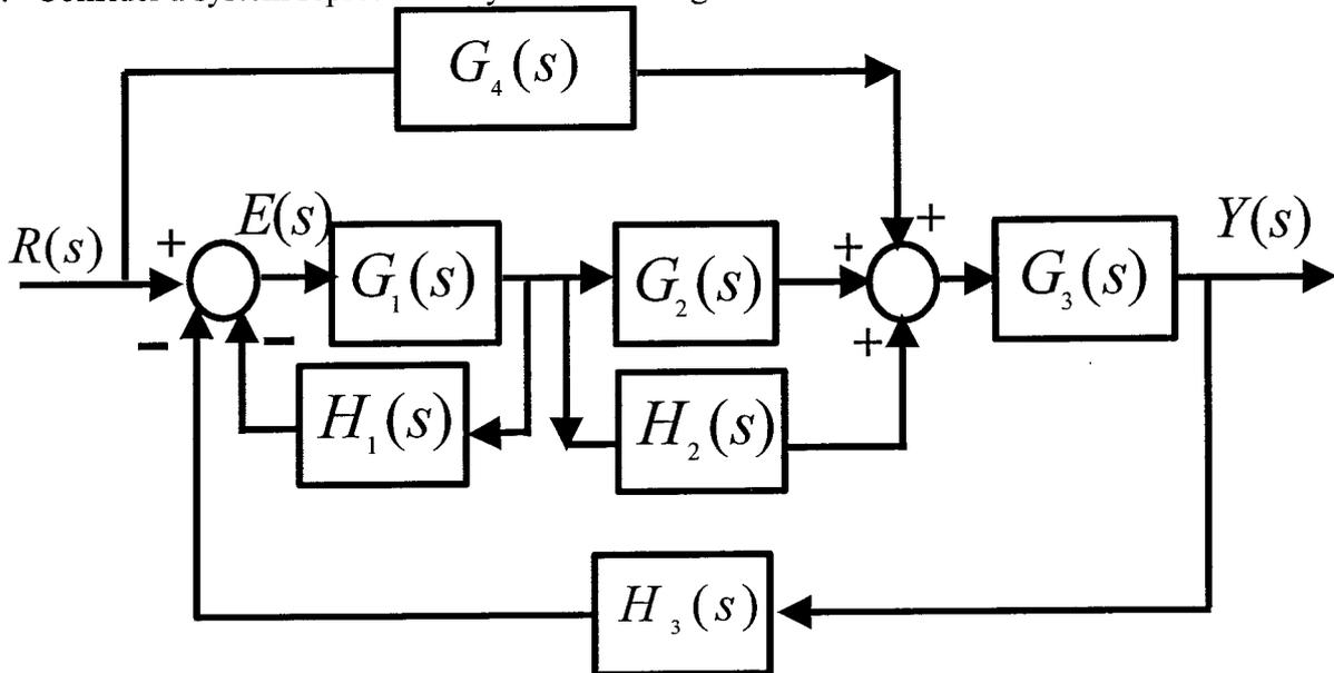
Find the closed-loop transfer function  $T(s)=Y(s)/R(s)$ .
